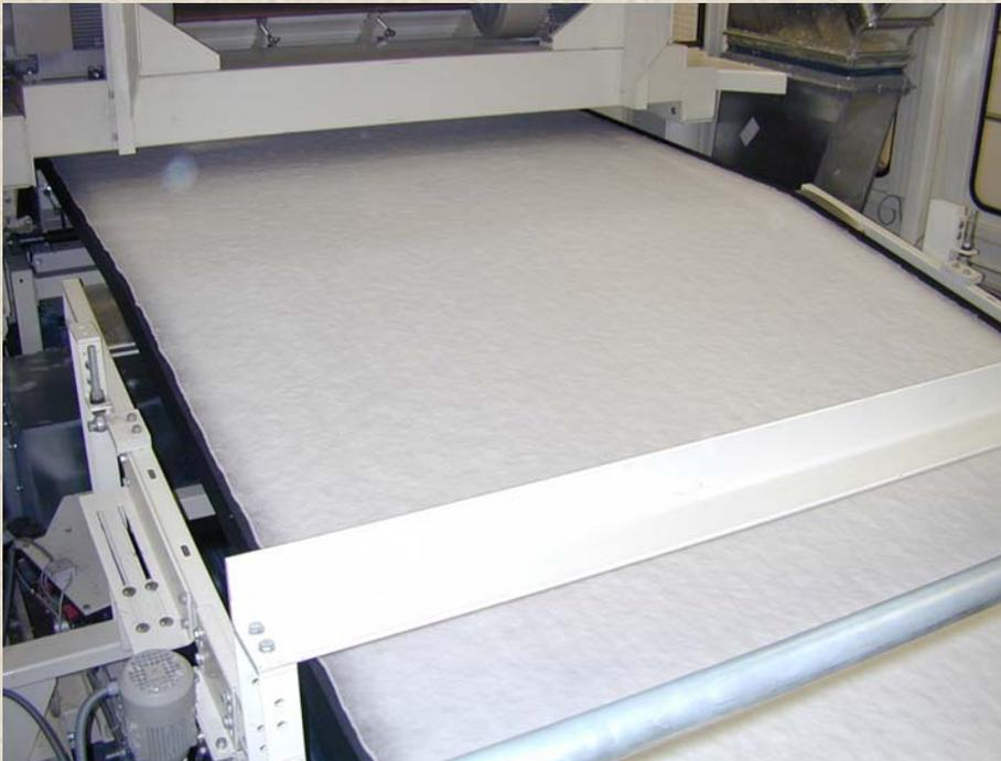
$m = 80 \text{ g/m}^2$ ;  $v = 35 \text{ m/min}$ ;  $P = 168 \text{ kg/h/m}$
